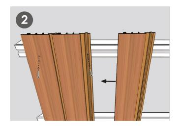
Insert further panels in the previous one and repeat this process until you reach the required width.
