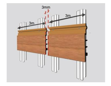
When connected to other surface e.g., concrete wall, an expansion spacing of 3mm is required.
