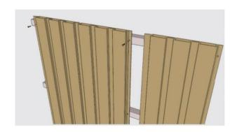
Insert further panels in the previous one and repeat this process until you reach the required width.
